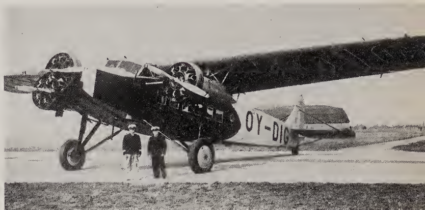
left The Fokker F.XX with Wright Cyclone engines, which appeared in 1933, was the most refined of the trimotor designs, with, for example, a retractable undercarriage. It carried twelve passengers
