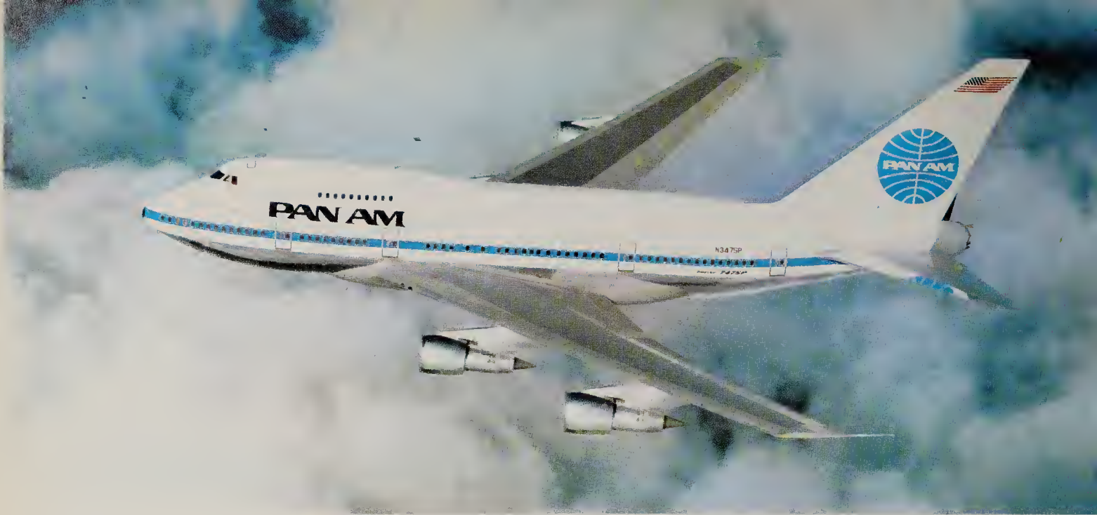
above Boeing 747SP is a short-fuselage version of the familiar 'Jumbo'
