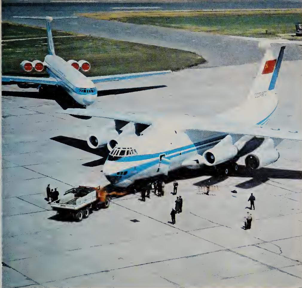
left Ilyushin Il-76 (foreground) was designed as a military transport, while the Il-62 (background) is a long-range airliner similar in configuration to the British VC-10
