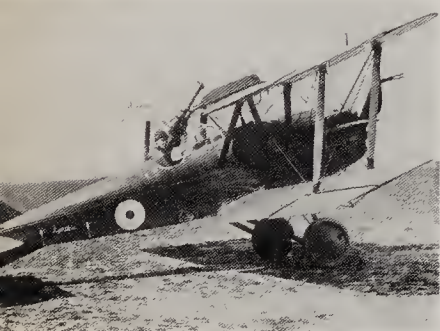
above An early production S.E.5 fighter showing its Lewis gun mounting
