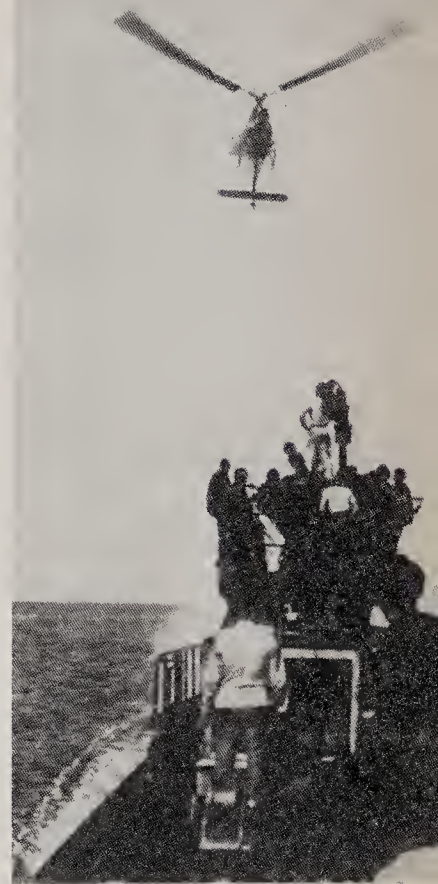
The Focke-Achgelis Fa 330 was the non-powered 'kite' helicopter glider for use from submarines
