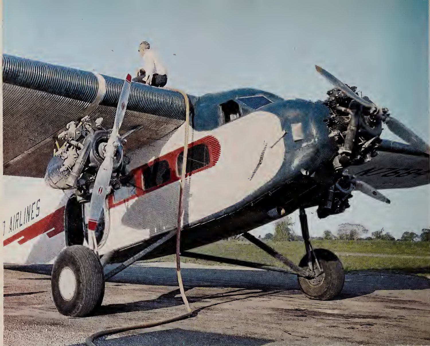
Ford Trimotor shown here being refuelled was still flying in regular airline service in the 1960s with an US internal line. It was rumoured that a Fokker was surreptitiously measured by Ford designers before the 'Tin Goose' was finalised
