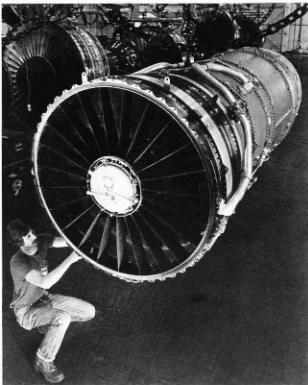
Pratt & Whitney's JT8D-200 series engine powers Continental Airlines' McDonnell Douglas MD-82 transports.
