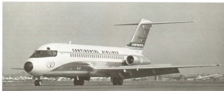
The DC-9-10C was a version of the Douglas twin jet, equipped with a large cargo door. It could quickly be converted from passenger to freight configuration. It entered service on April 10, 1966, replacing the Viscounts.
