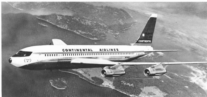
The Boeing 720B, a smaller version of the B-707, was equipped with fanjet engines, and went into service on June 3, 1962.
