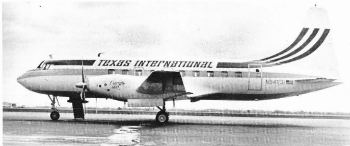
T.T.A.'s selection for the DC-3 successor was the Convair 600. This was basically the Convair 240, but re-engined with Rolls-Royce Dart turboprops. It is seen here in Texas International colors.
